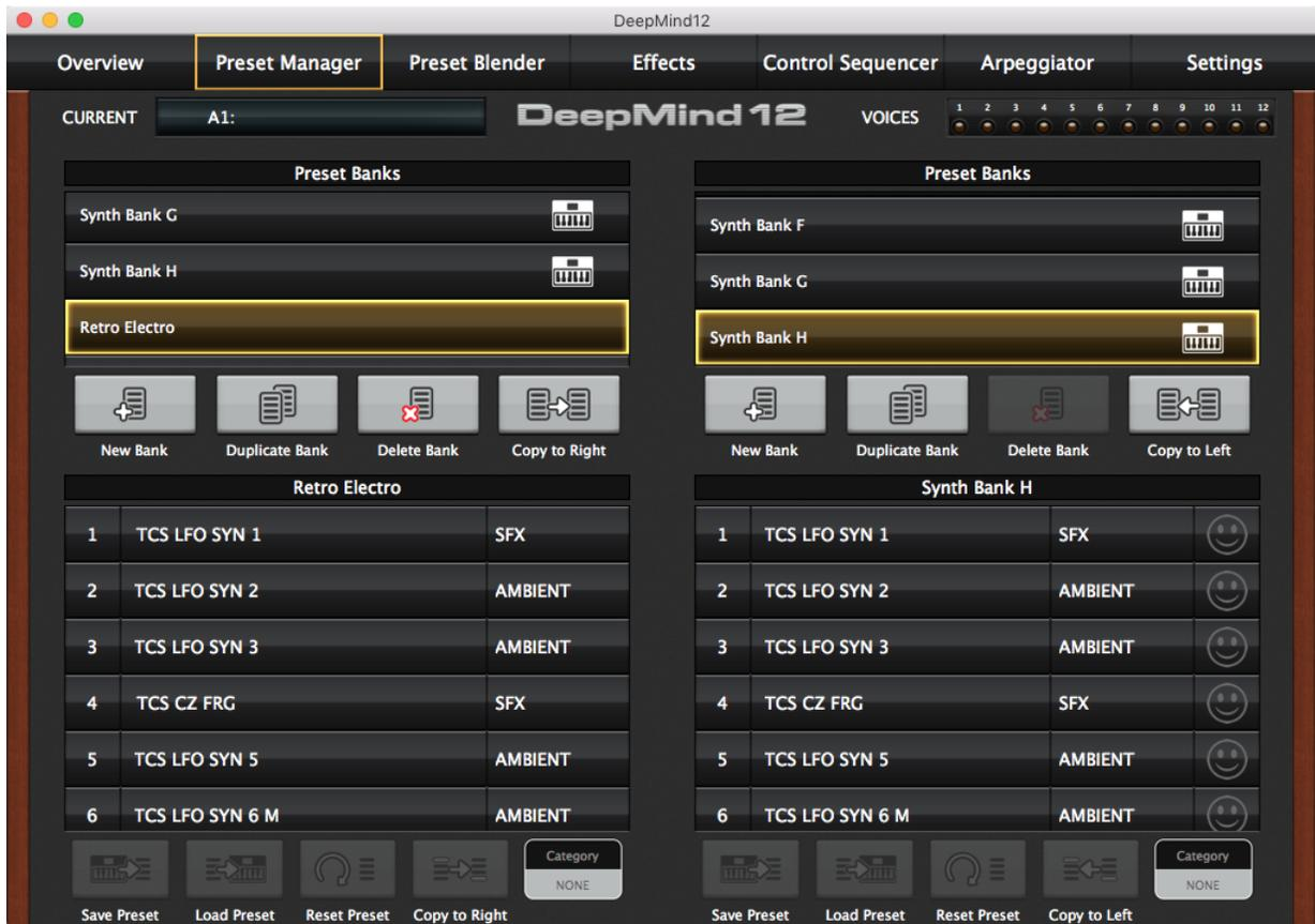
To import the sound bank into the DeepMind, select which bank you wish to import to on the right-hand side and then click the 'Copy to Right' button. Please ensure your DeepMind remains connected via USB until the import procedure has been completed.
